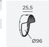
Partial rotatable visor, to assist with the shielding of any directional glare.
