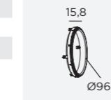
Primary ring that enables the housing of any accessory to be fixed on the front of the standard ring.
