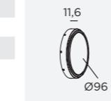
Rotatable lens to allow the elliptical deformation of the beam amplitude and variable illuminated characteristics, co-dependent on the chosen optical combination.
