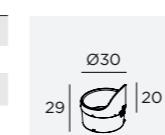
Snap-on accessory for the partial and directional reduction of glare. Can rotate of 360°. Replaces the ring supplied as standard.
