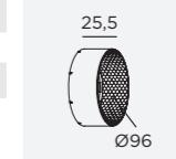
Omnidirectional glare reducer, to assist in shielding any radial glare disturbances.
