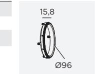
Primary ring that enables the housing of any accessory to be fixed on the front of the standard ring.
