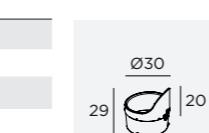
Snap-on accessory for the partial and directional reduction of glare. Can rotate of 360°. Replaces the ring supplied as standard.
