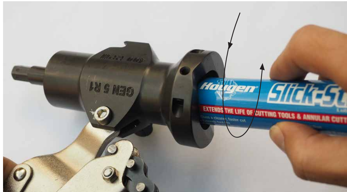
Fig. 5.1 IMPORTANT! Lubricate the cutters before drilling each hole. A light twist action will supply a sufficient amount.
