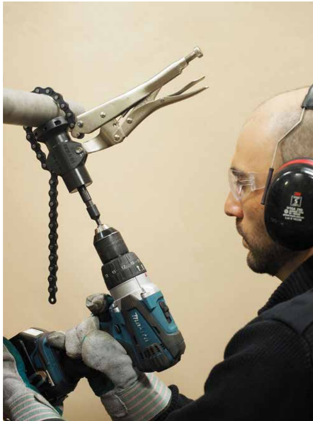
Fig 8.1 Do NOT force / push the drill. Use light pressure only to keep the socket engaged.
