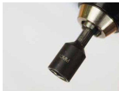
Above: Check the 10mm driver bit is secure
