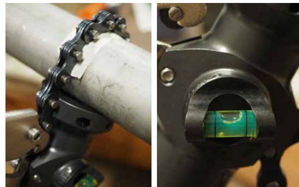
Fig. 6.2 - 6.5 align clamp body with the tape and engage the chain hook and clamping chain. Ensure the spirit level bubble remains centred
