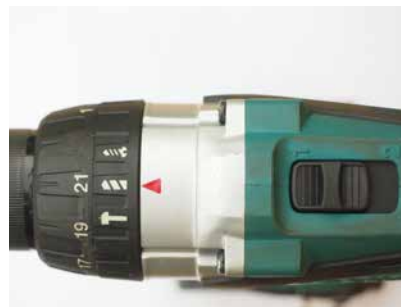
Above: Our example drill is set to: "Drill"; high torque; and LOW speed (1)
