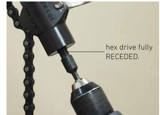
Fig. 8.2 STOP drilling once the hex drive has fully retracted inside the Drill Jig.
