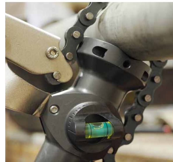
Above: The drill Jig's spirit level bubble should be centred before drilling to enable consistent angle drilling at your set angle.
